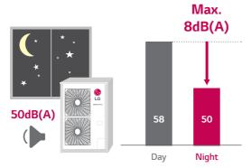
\* Normal mode noise level (10HP): 58dB(A) \* Night 3 step noise level (10HP) : 56dB(A), 53dB(A), 50dB(A)
